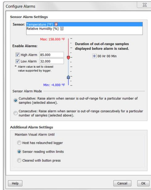
3. Select the High Alarm checkbox if you want an alarm to trip when the sensor reading rises above the high alarm value. Type the reading next to the High Alarm checkbox or drag the red upper slider in the Configure Alarms window.
