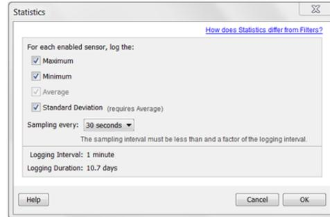
3. Set the sampling interval, which must be less than and a factor of the logging interval. Choose either a preset sampling interval or select Custom and enter your own sampling interval. Keep in mind that the more frequent the sampling rate, the greater the impact on battery life.
