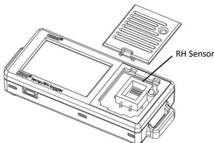
2. Use needle-nose pliers to remove the RH sensor from the board inside the logger case and discard it.
